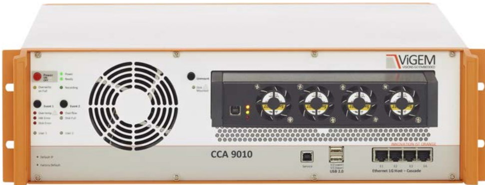
Front view: Removable data storage and data outputs
