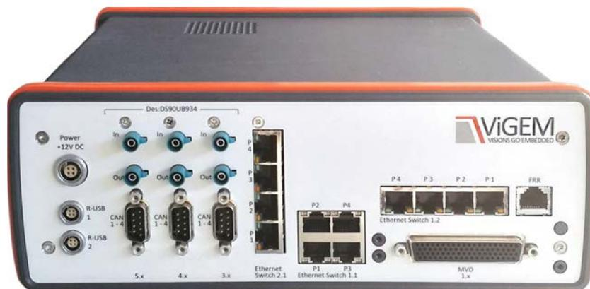
Rear view: Data inputs (configuration example)
